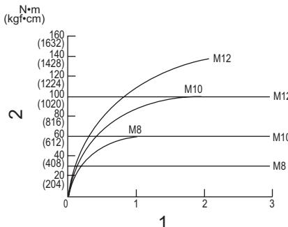
1. Fastening time (second) 2. Fastening torque
