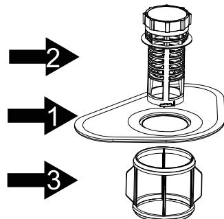
Check the condition of the filters after each washing.
