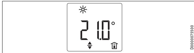
The standard display is continuously displayed. If no user action is performed for longer than 20 seconds while in the menu, the device automatically switches to the standard display.
