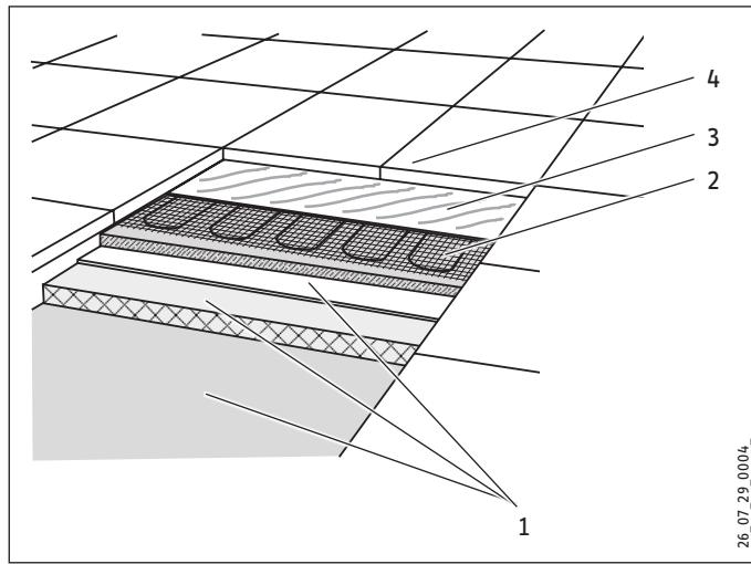
1 Substrate with thermal insulation
