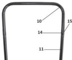
Using the included M6x30 bolts (14) and M6 nuts (15), connect the bottom part of handle A to the bottom part of handle B, and then connect them to the middle parts of the handle (11).
