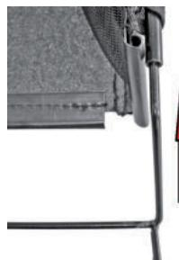
Connect the bottom and sides of the grass catcher net (16) to the grass catcher frame (17).
