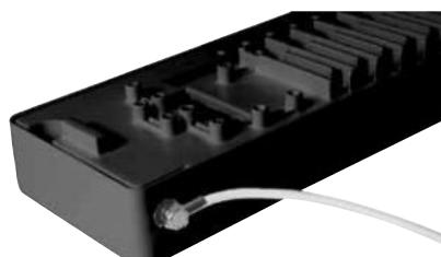
1. Remove the plastic cover from the antenna connection.
