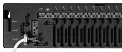
1. Connect an external ON/OFF switch to the terminals for Heating & Cooling. When this switch is closed (ON) the system will switch from heating to cooling.
