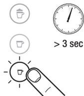
**3** Release button when desired volume is reached. Coffee volume is now stored for the next coffee preparations. Button blinks 3 times to confirm the new coffee volume.
