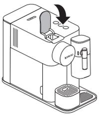
**7** To prepare a second beverage, remove the milk container lid and fill the milk container up. Do not exceed the MAX level. Repeat operations 1 to 6.
