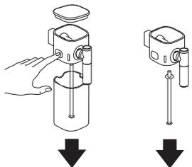
**2** Position the milk spout vertically to disassemble and to reassemble.
