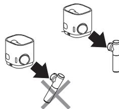
**3** Press the button on the side of milk jug and pull to unlock the connector.
