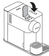
**3** Empty the drip tray and the used capsule container. Fill the water tank with 100 ml of **Nespresso** descaling agent (1 pouch). Add water up to the descaling mark on the water tank (~500 ml).
