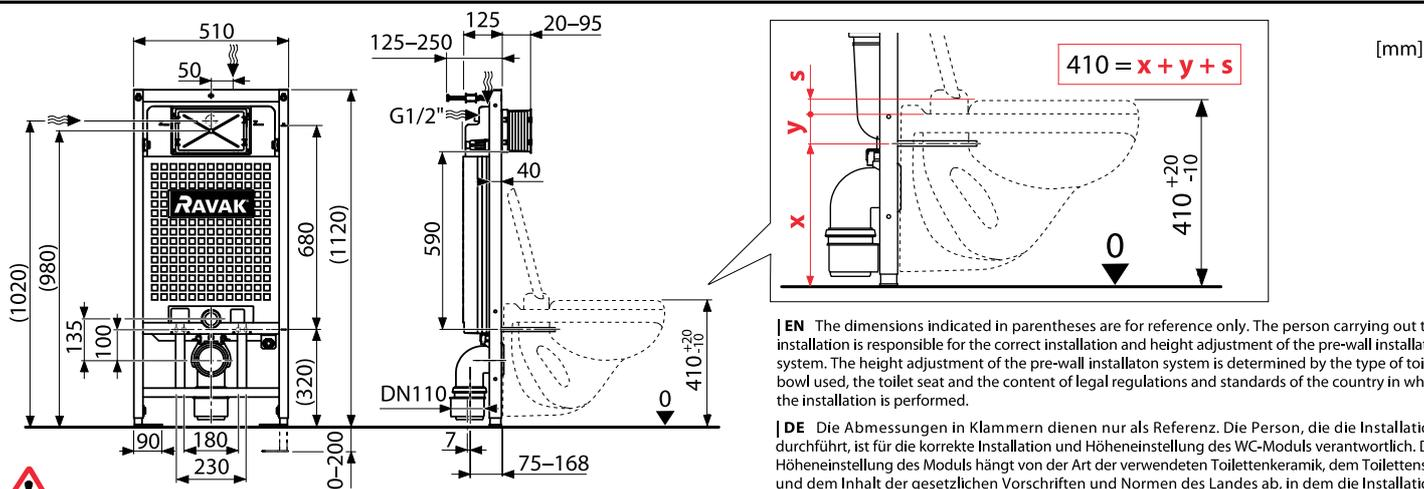
**EN** The dimensions indicated in parentheses are for reference only. The person carrying out the installation is responsible for the correct installation and height adjustment of the pre-wall installation system. The height adjustment of the pre-wall installation system is determined by the type of toilet bowl used, the toilet seat and the content of legal regulations and standards of the country in which the installation is performed.
