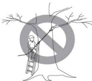
Never work from a ladder or other unstable equipment while working with a chain saw. Always grasp the chain saw with both hands. While cutting, apply firm and continuous pressure on the chain saw but do not try to force the chain saw through the wood being cut. Do not use the chain saw for cutting branches having larger diameter than the length of the guide bar.
