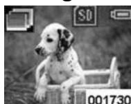
In Capture Mode, press Power Button once brings to Menu Mode . Press Left Button **twice** to see the "Blast icon" . Then, press Shutter Button to return to the Capture Mode. You can see the "Blast" icon stays on screen's upper-left corner. Now your camera is ready to take three pictures in a row after pressing the Shutter button.
