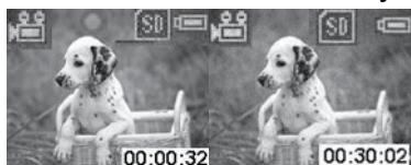
During recording, you can see recorded time (00:00:32) on screen's lower-right corner. Press Shutter Button again to stop video recording. **Caution!** When SD/MMC card is full, “**CARD FULL**” message appears on the LCD screen. Please download or erase pictures/videos to free up memory space.
