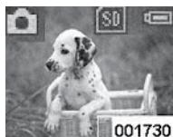
After turn on the camera, objects captured by the lens can be seen on the LCD screen. Your camera is in Capture Mode and ready to take picture. Aiming at the object and then press the Shutter Button once. The LCD screen will turn into dark and then shows the picture taken for ~ 1 second. The camera will return to capture mode and ready for taking next picture. On screen's lower-right corner, it shows number (001730) of photos left to take.
