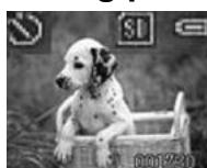
In Capture Mode, press Power Button once brings to Menu Mode . Press Right Button once to see the "self-timer" icon . Then, press Shutter Button to return to the Capture Mode. You can see the "Self-Timer" icon stays on screen's upper-left corner. Now you can take picture with Self-Timer. Picture will be captured 10 seconds after pressing the Shutter button.
