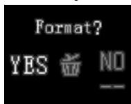
To format the SD CARD, press the Playback Button to enter Playback Mode. Press the Power Button twice, you can see the LCD screen as shown on the right. Press the Left button to select YES. Then press the Shutter Button to format the SD CARD. Once SD card is formatted, "NO FILE" is shown on the screen and you can press Playback Button to return to Capture Mode.
