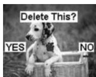
To delete pictures, press the Playback Button to enter Playback Mode. Press the Left or Right Button until the photo to be deleted is displayed. Afterwards, press the Power Button once. You can see the LCD screen as shown on the right. Press the Left button to select YES, then press the Shutter Button to delete the picture. The camera will return to Playback Mode once picture is deleted. You can press the Playback Button again to return to the Capture Mode.
