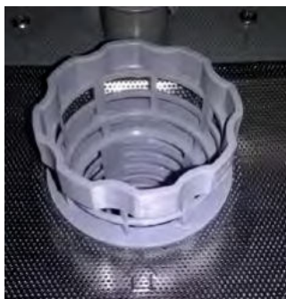
Poorly secured filter
