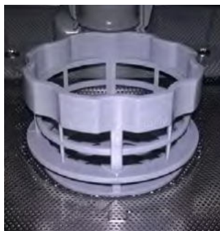
Properly secured filter
