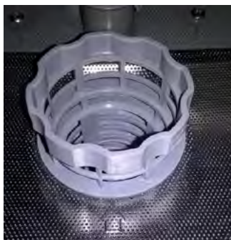
Poorly secured filter
