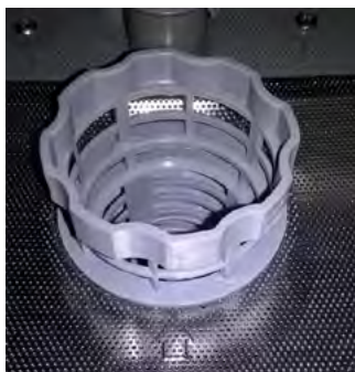
Poorly secured filter
