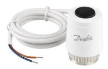
Danfoss thermal actuator TWA-Z is used with Danfoss automatically balanced combination valves type AB-QM. The actuator can be controlled with an on/off controller, pulse width modulation (PWM), or switch.
