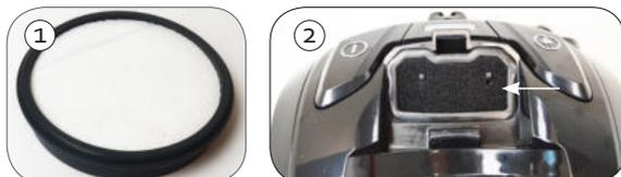
3. On the back of the appliance there is a grille for the hepa filter. This can be easily removed by pushing the clip of the grille to the right, and taking the grill out of the appliance. Take the hepa filter out of the appliance by pushing the clip to the left.
