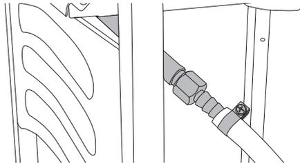
3. Make sure that the gas control knobs are set to **OFF**.
